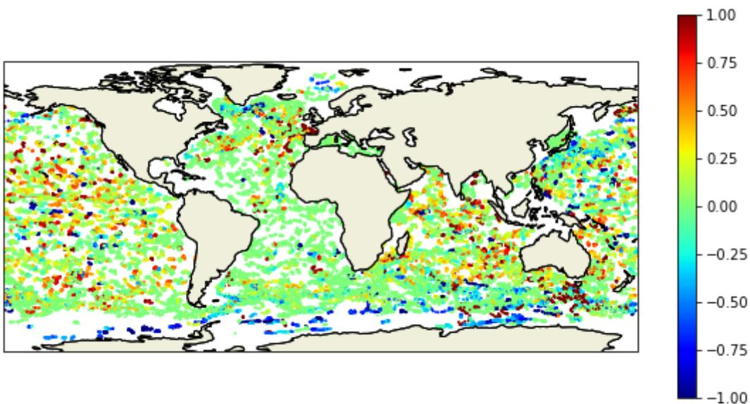
**SLA interpolation on Argo float positions**
