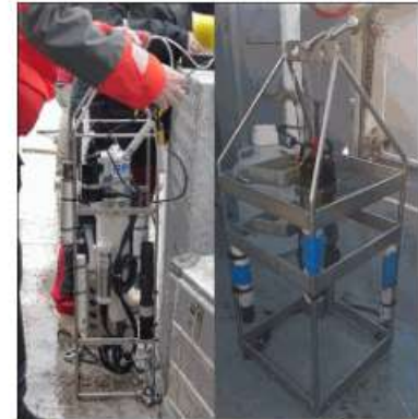
Nicolas Dubosq (left) - University of Bordeaux (right) The multiparameter probes SeaBird SBE-19plus (left), Wimo Plus (right) and autonomous sensors fixed on the supports
