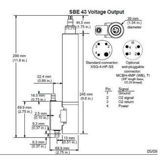
Clark-cell sensor (electrochemical) Most common sensor used to measure DO concentrations during CTD profiles (fast response)
